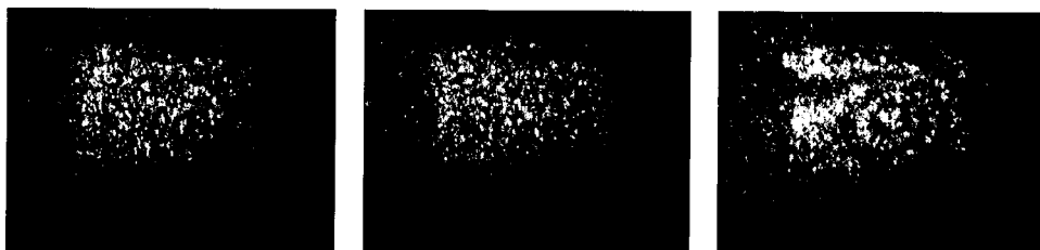
Fig. 13 DMD reconstruction of an Al plate. Left: initial state; middle: loaded state; right: holographic interferogram.
